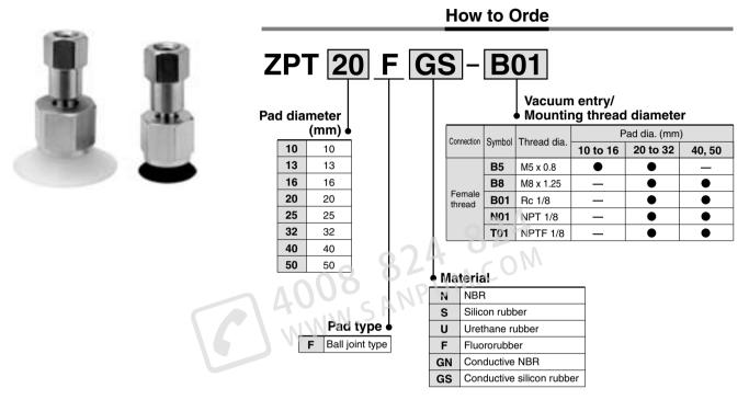
Note) Pads are exclusively ball joint type and are not interchangeable with other pads.
