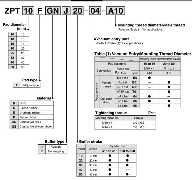
Note) Pads are exclusively ball joint type and are not interchangeable with other pads.
