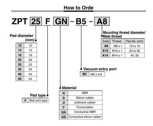
Note) Pads are exclusively ball joint type and are not interchangeable with other pads.
